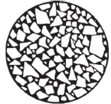
Figure 23.1 The type of structure in a tungsten carbide/cobalt cermet. Particles of tungsten carbide (white) in a cobalt matrix (black) ( \times 1000 ).
